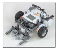
Line Sensing Pusher Driving Base + Pusher + Light Sensor
