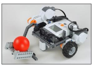
**Line Following Forklift**Robot Base + Forklift Arm + Light Sensor
