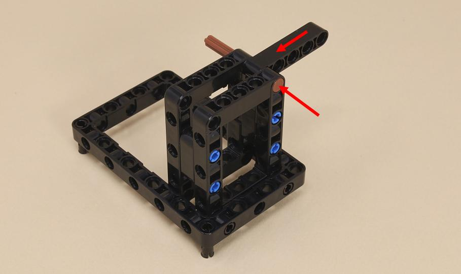
Pull the claw motor wire down and out of the way, and slide the arm onto the axle.
